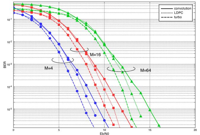
Fig. 1. BERs for BICM-OFDM using LDPC code, turbo code, and convolutional code with random interleaver over frequency-selective Rayleigh fading channels.
