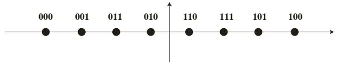
Fig. 3. Gray labeling for the in-phase of 64QAM (8-ASK).
