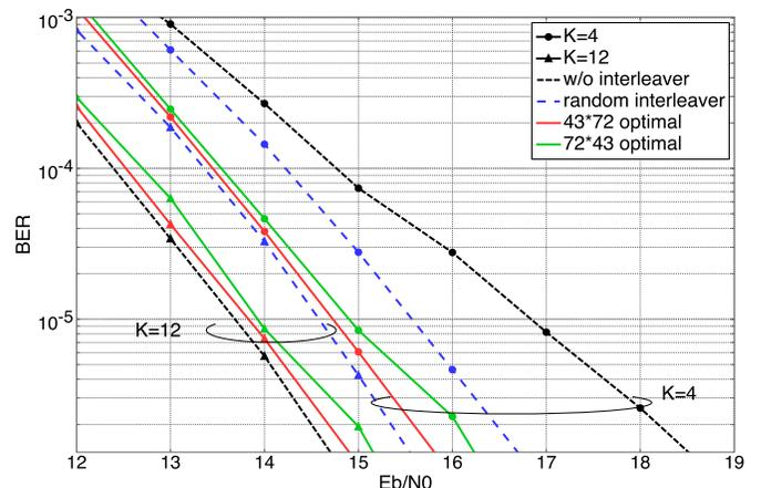
Fig. 8. BERs for BICM-OFDM for  $M = 256$  with convolutional code with random interleaver, optimal interleavers, and without interleaver over Ricean fading channels.
