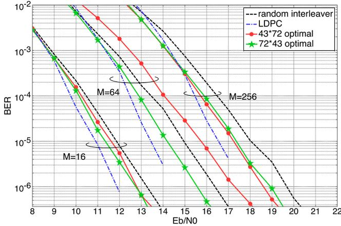
Fig. 6. BERs for BICM-OFDM with convolutional code with random interleaver and optimal block interleavers and LDPC code over Rayleigh fading channels with equal delay intervals.
