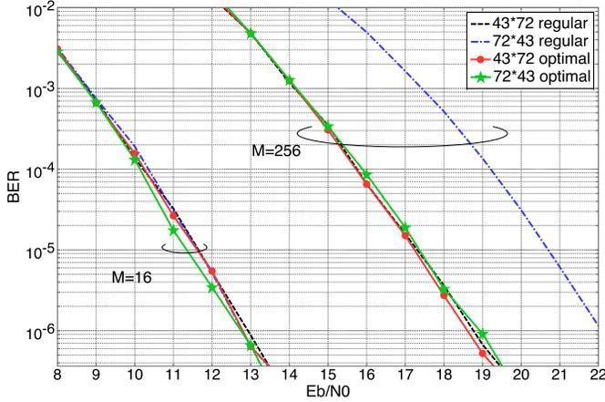
Fig. 5. BERs for BICM-OFDM with convolutional code with regular and optimal block interleavers over Rayleigh fading channels with equal delay intervals.
