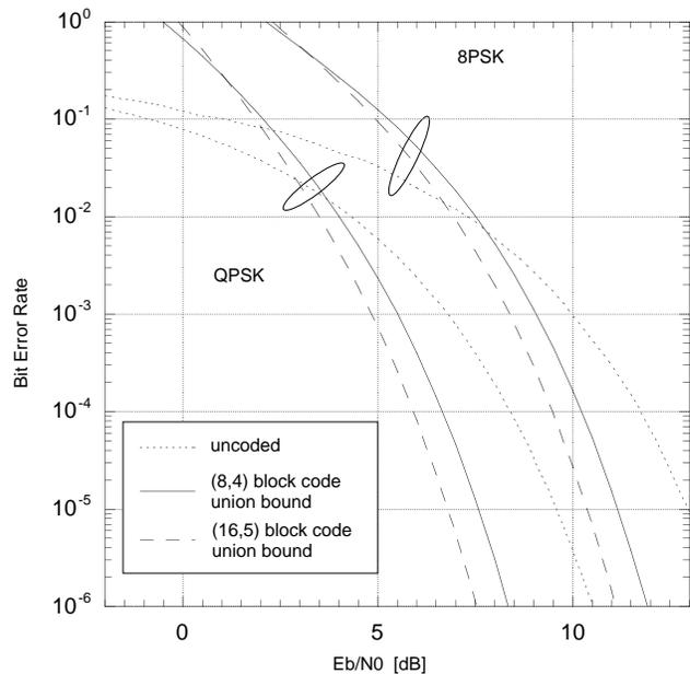
Fig. 4: Union bound of the block codes over AWGN channel
