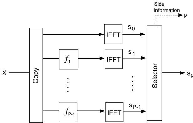
Fig. 2: An example of selection-based peak-power reduction schemes
