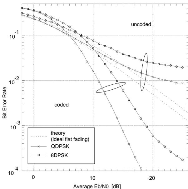
Fig. 5: Performance of the (16,5) block code over frequency-selective fading channel ( $N = 16$ , PAPR=3 dB)
