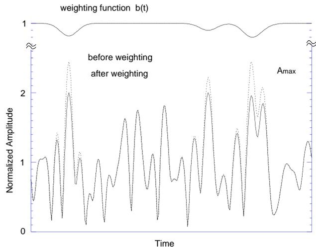
Fig. 1: Peak power reduction by weighting function ( $N = 128$ ,  $A_{max} = 2.0$ )
