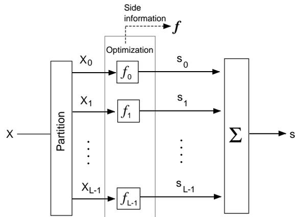
Fig. 3: An example of optimization-based peak-power reduction schemes
