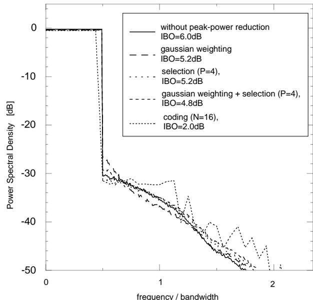
Fig. 6: Spectra of peak-reduced OFDM signals over SSPA channel ( $p = 5$ ),  $N = 128$  (except for coding  $N = 16$ )
